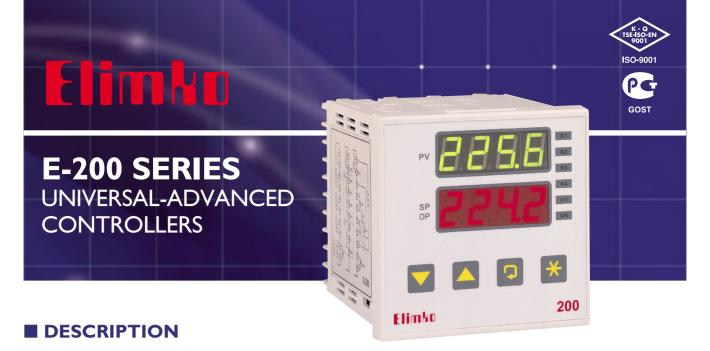
E-200 Series universal-advanced controllers are designed using new generation micro-controllers. Unit dimensions are 96x96mm, conforming to IEC 668. E-200 Series has a 2x4 digit LED display range from -1999 to 9999 and configurable universal inputs (R/T, T/C, mV, mA) with 16 bit resolution and ultra low calibration drifts with environmental conditions.
