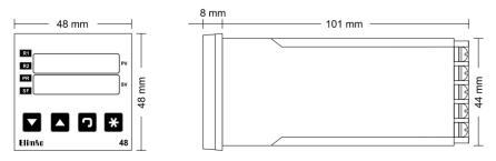
Panel cut-out =  $45 \times 45 \text{ mm}$
