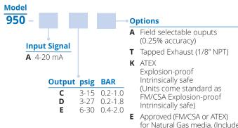
Approved (FM/CSA or ATEX) for Natural Gas media. (Includes tapped exhaust and factory sealed conduit assembly)
