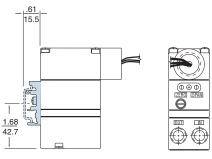
DIN Rail Kit suitable for EN-50035, EN-50045 and EN-50022 Rails
