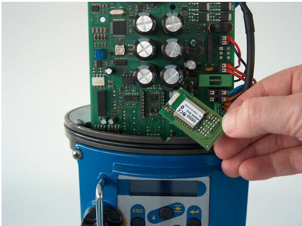
After insertion of the Bluetooth module has the actuator is ready immediately to communicate with any Bluetooth-enabled notebook-PC in the field. No additional software needs to be installed. The parameterisation software PSCS remains the same and offers identical functions as does a conventional connection via cable or by a field bus.
